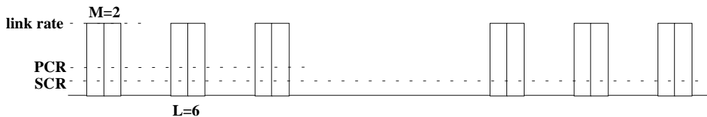
Fig. 3. A near worst case traffic pattern with given PCR, SCR, SDVT and IBT; M = the maximum number of consecutive cells; L = the maximum burst size in cells.
