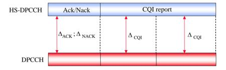
HS-DPCCH introduces an overhead that can be taken into account as an offset to be added to the target DCH E<sub>b</sub>/N<sub>0</sub>, i.e.
