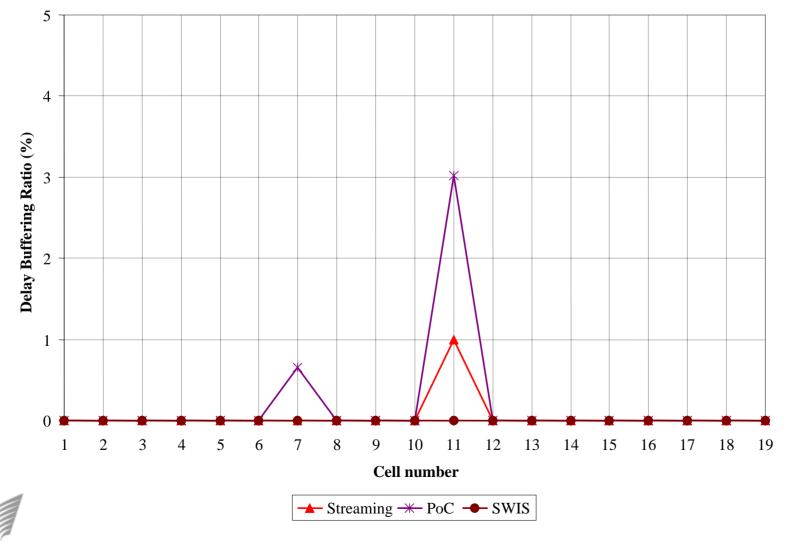
The tolerance of streaming users is higher than for PoC
