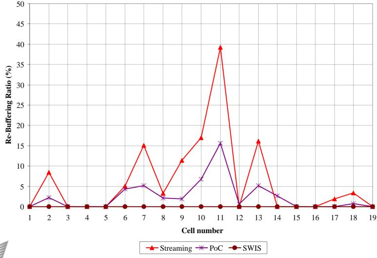
The rebuffering ratio is correctly higher for streaming
